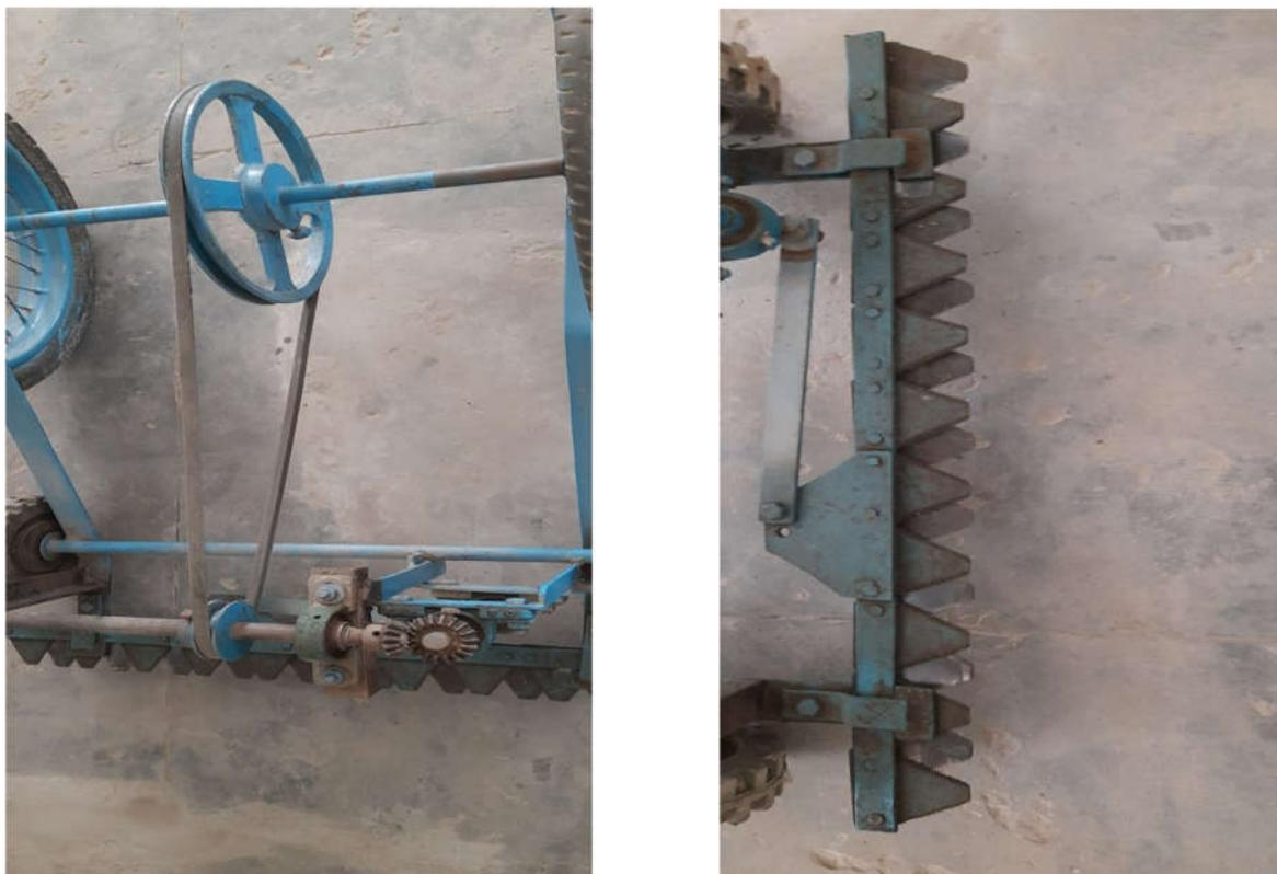
**Fig. 4.2:** Power Transmission and Cutting Arrangements of Machine
