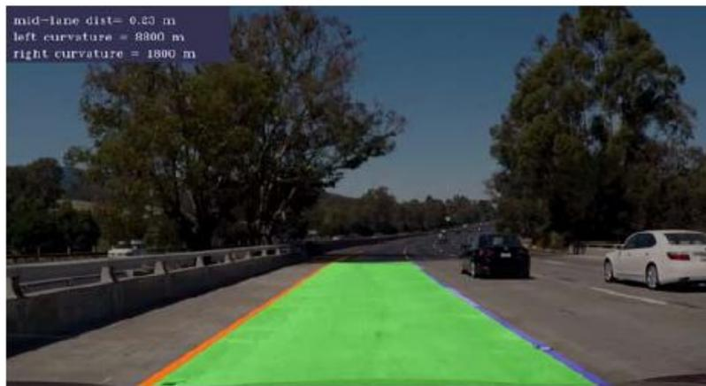
Fig. 4. Image of Lane Detection
