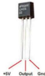
FIG 1: Temperature Sensor.
