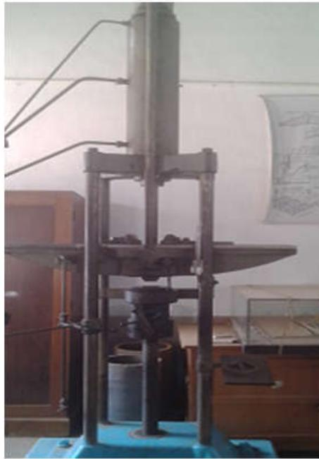
Flexure strength testing machine
