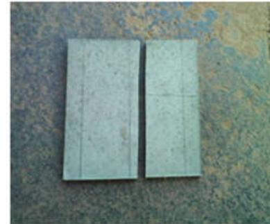
Tile after flexure test.
