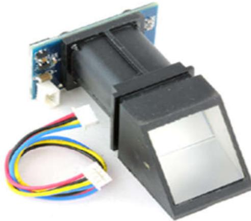
Figure 3.4: Fingerprint Module
