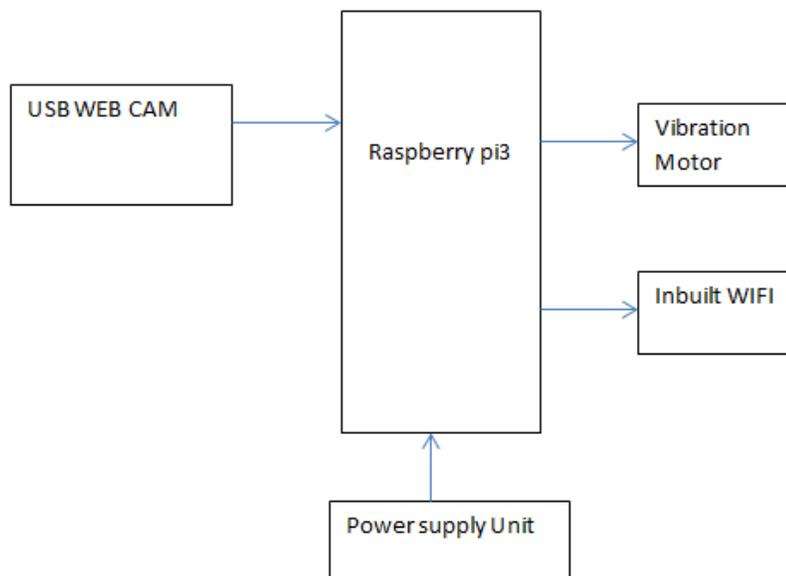
USB WEB camera is attached to Raspberry pi for live face recognition purpose. If captured face is matched with predefined stored data base, automatically vibration motor will on for door open demonstration purpose. If captured image is not in trained database, a warning message will be forwarded to owner mobile android app through internet of Technology using inbuilt WIFI module.
